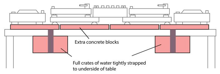
Here, the vibration of the tabletop itself is first damped by strapping heavy stuff to it (concrete and/or water crates); then, the first technique is applied on top of that.
