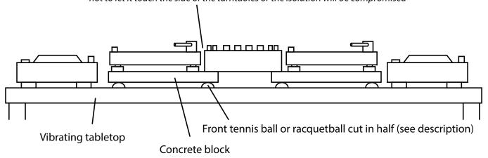
In the above setup, the heavy concrete blocks are isolated from the vibrating table by the rubber balls, providing a vibration-free surface for the turntables to sit on.
